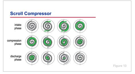
During the first full revolution of the shaft, or the **intake phase**, the edges of the scrolls separate, allowing the refrigerant vapor to enter the space between the two scrolls. By the completion of first revolution, the edges of the scrolls meet again, forming two closed pockets of refrigerant.
